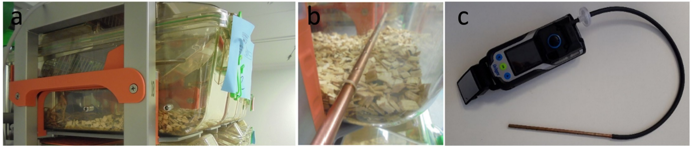
Fig 1. a) Modified IVC GM500 cage with holes drilled in the long side, sealed with screws and nuts inserted into the DVC ® rack. b) Lateral view of the modified IVC GM500 cage with the NH 3 detector probe inserted across the width of the cage to perform the ammonia measurement. c) Dräger X-am ® 8000 device with a 40 cm long rubber tube, dust filter and copper probe.
