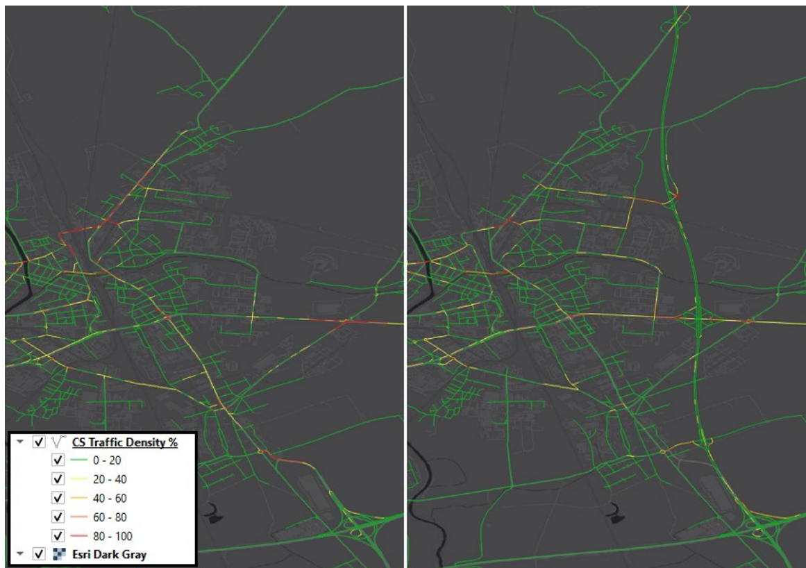
Figure 70 Comparison of roads, exported from the model of Olomouc and imported to QGIS, and their traffic density before (left) and after (right) constructing the highway bypass.
