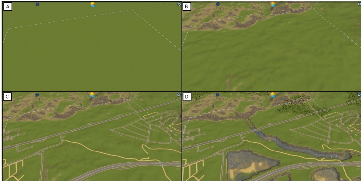
Figure 18 Creation of the base model of Svit from geographical data using the GeoSkylines methods. A: an empty map after opening the map editor, B: the map after uploading the terrain, C: the map after generating the road network, D: the map after generating basins with water sources and tree coverage.
