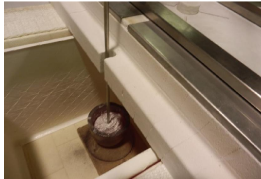
Figure 68 mixing shaft and impeller
