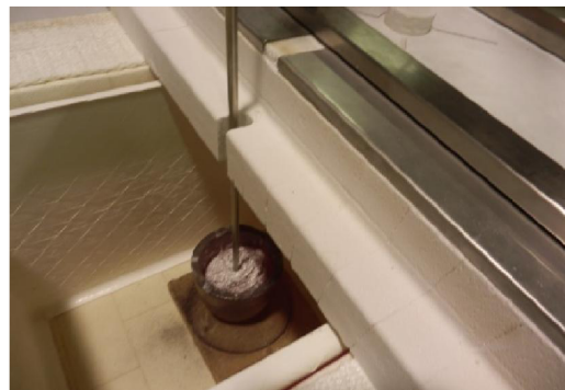
Figure 68 mixing shaft and impeller
