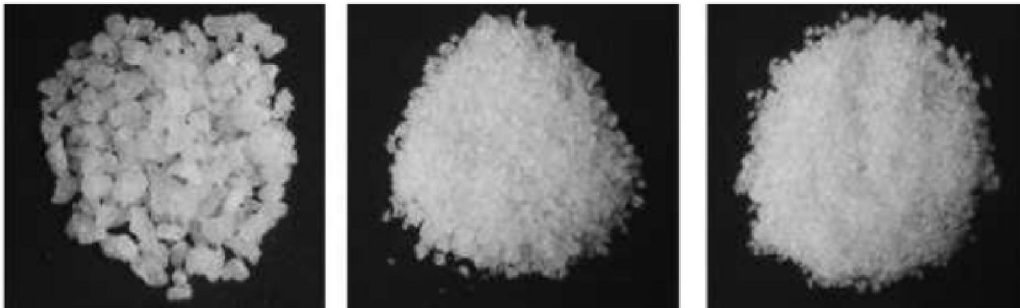
Figure 70 different particle size used for NaCl place holders for the metal foam, 9 mm left, 6 mm middle and 4 mm right [77]
