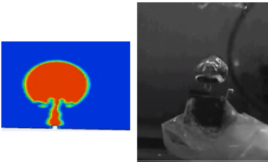
Figure 53 simulation vs speed camera shape bubble, nozzle exit
