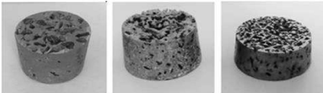
Figure 69 samples produced from the procedure: 9 mm place holder particle size on the left, 6 mm in the middle and 4 mm on the right [77]
