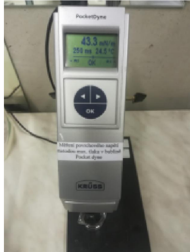
Figure 21 measuring Surface tension
