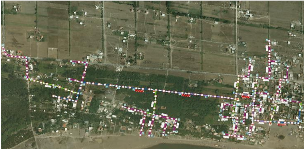
Photo 5.1. Sewage Collection System of Velipoje
