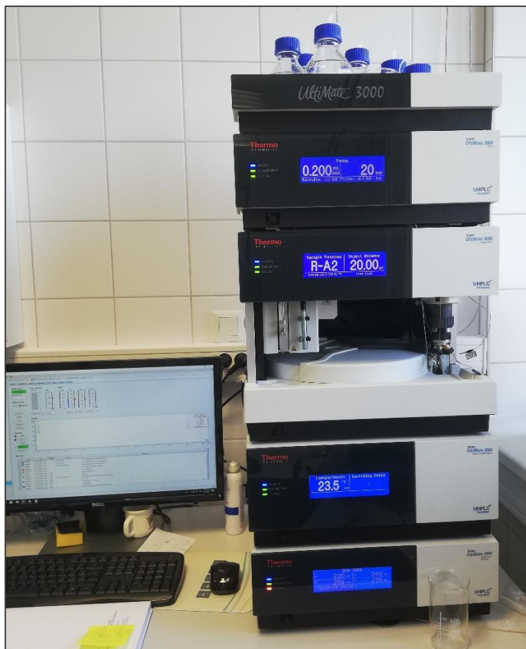
Figure 10: High-Performance Liquid Chromatography (HPLC) Coupled with a Diode Array Detector System Ultimate 3000 (Thermo Scientific, Pragolab, Czech Republic)
