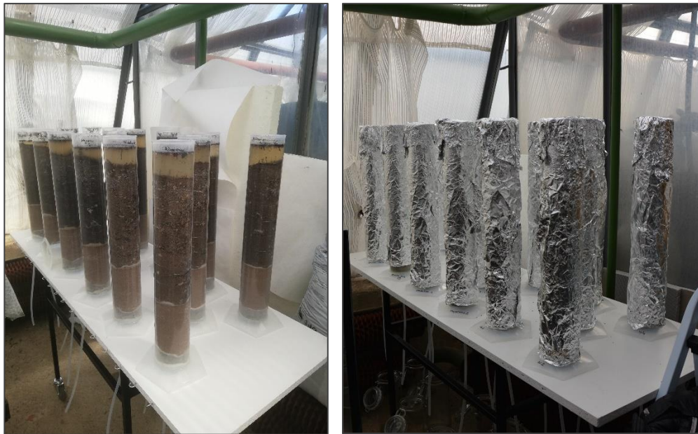
Figure 6: The picture of the columns in the greenhouse. On the right, the columns after covered with aluminum foil.
