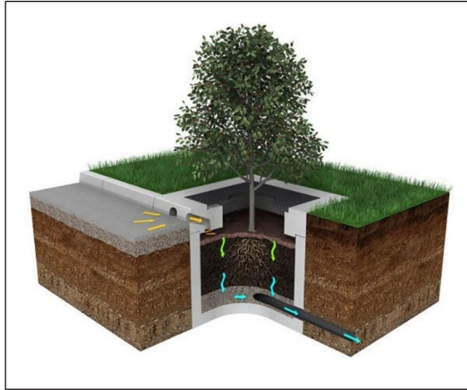
Figure 1: Biofiltration System Designed for Treatment of Stormwater
