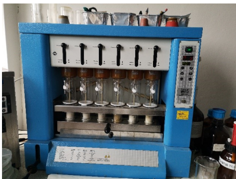
SER 148 apparatus – crude fat analysis
