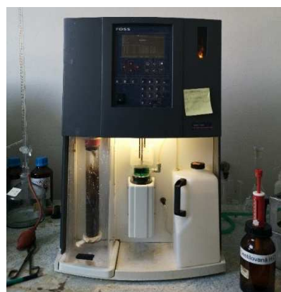
Kjeltec 2400 apparatus – protein analysis, Digestion unit – MB 442 (FOSS, Denmark)
