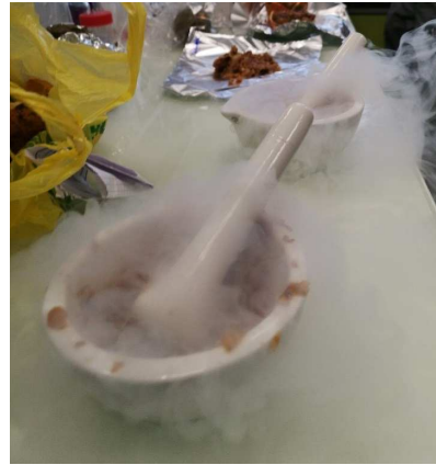
Grounding fruit pulp together with nitrogen in a mortar with pestle
