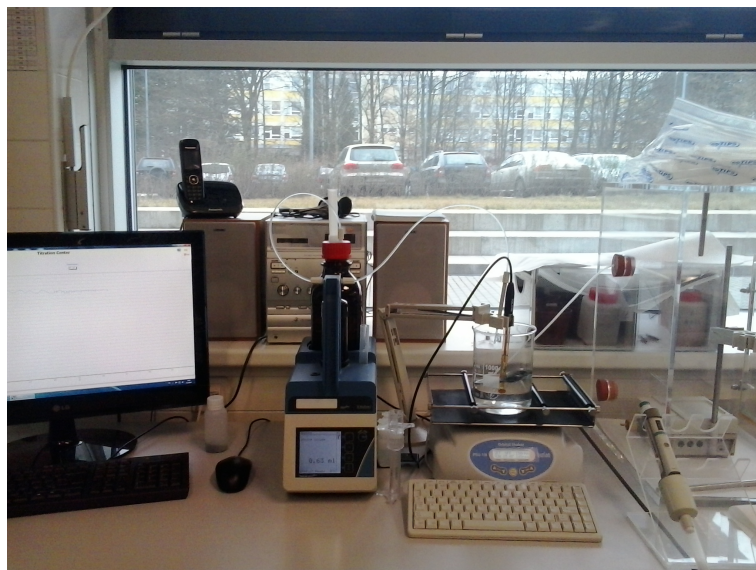
FIGURE C.1: Pb(II) and biochar solution agitation – for sorption.
