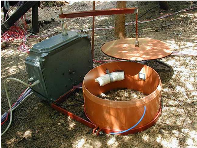
Fig. 8: Chamber for continuous measurement of soil CO 2 efflux in the spruce forest.
