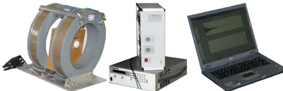
Fig. 21: The small NMR experimental system. Helmholtz coil (left hand side), electronics (above) and current source (bottom) (in the middle), and control unit – PC (right hand side).
