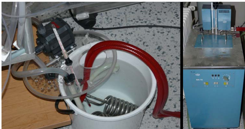
Fig. 14: Water reservoir (left hand side) – the bucket with acrylic lid, in which is a thermometer. Small pump Eheim 1048 is mounted on the lid. Two spirals are connected by red hoses with Ultra-Kryostat MK 70 (right hand side), which works as a cooler.
