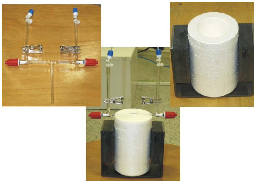
Fig. 35: Storage system for frozen xenon.
