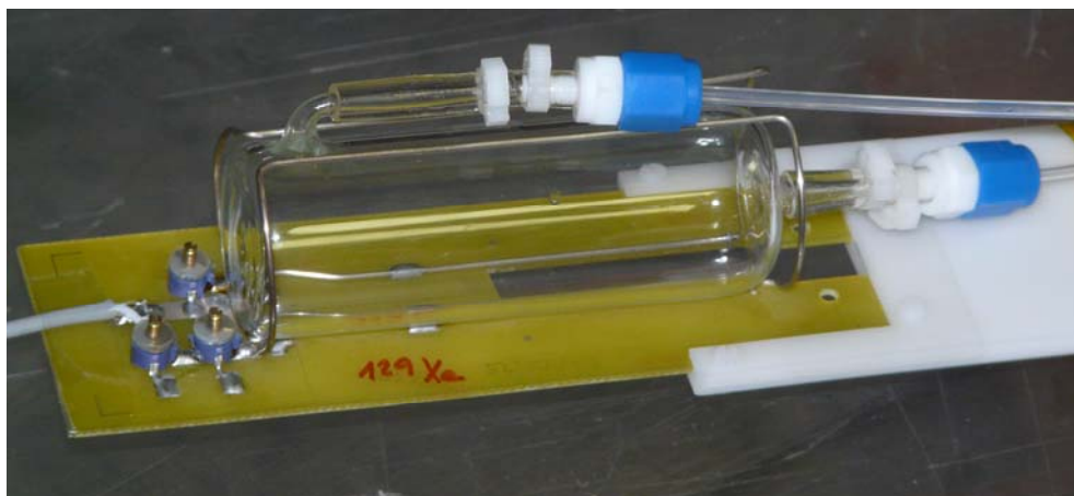
Fig. 19: Small ^{129}\text{Xe} saddle RF coil with a sample.
