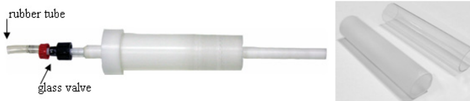
Fig. 36: Delrin shell with valve. On the right hand side are shown glasses samples.
