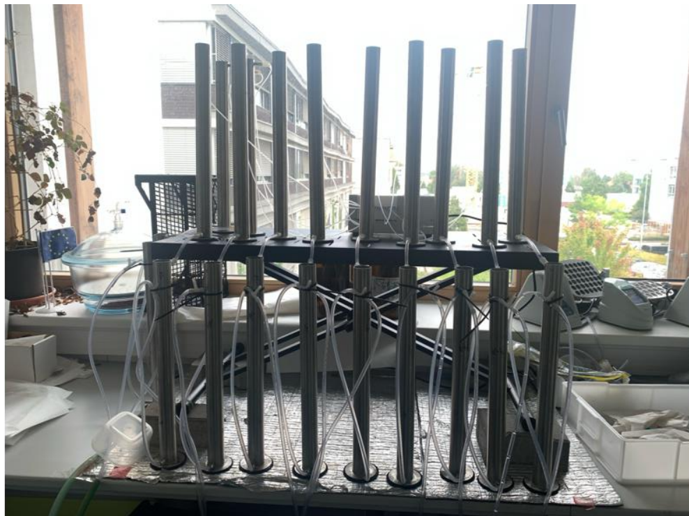
Fig. 3. Experimental biofilter columns of stage 1.
