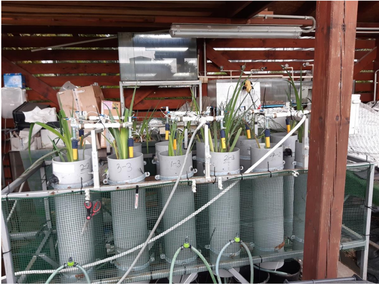
Fig. 5. The experimental set-up of the vertical-flow constructed wetlands.
