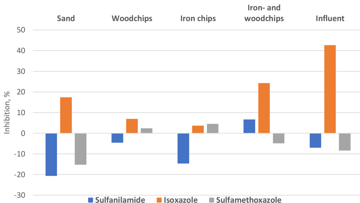
Fig. 11. Influent and effluent ecotoxicity determined by the Microtox bioassay ( Aliivibrio fischeri ).
