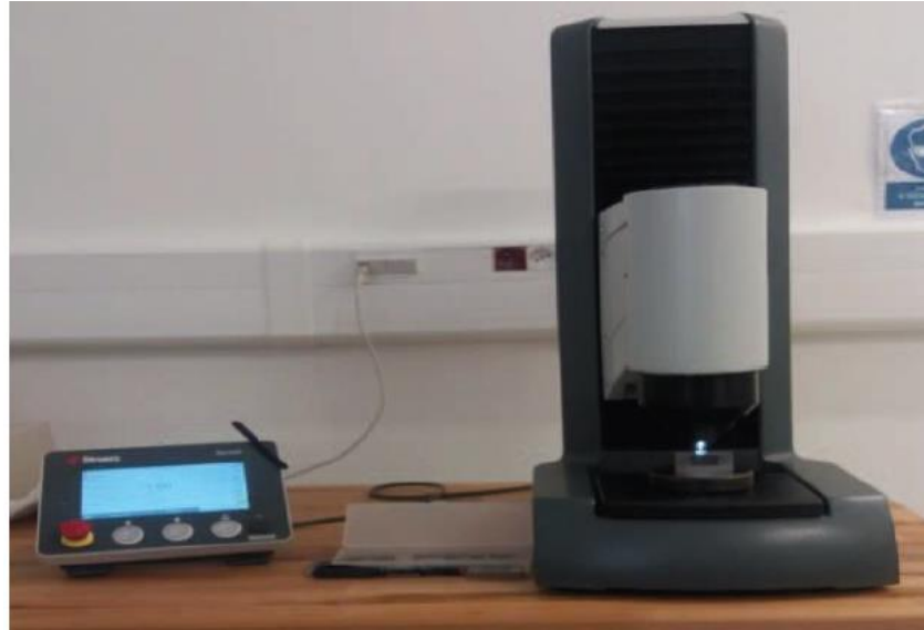
Figure 5.3 Vickers's Hardness Test in Laboratory of CULS, Faculty of Engineering, Department of Material Science and Manufacturing Technology
