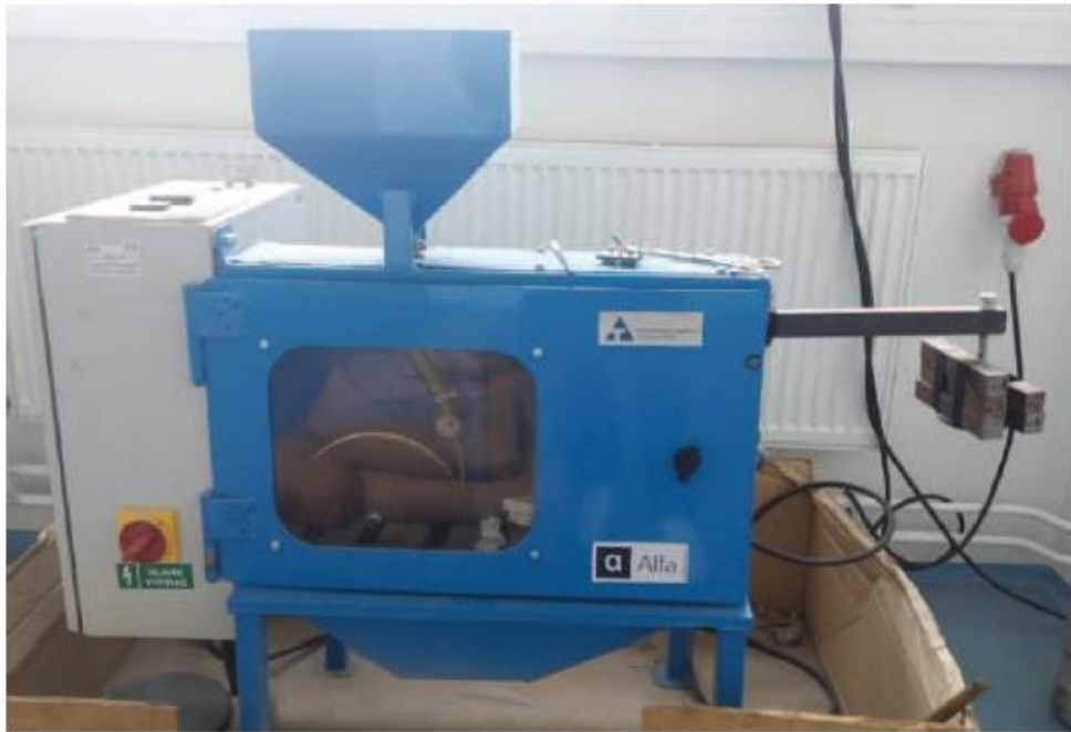
Figure 5.2 Standard test machine for measuring abrasion using the dry sand/rubber wheel device (ASTM G65), CULS, Faculty of Engineering, Department of Material Science and Manufacturing Technology's Laboratory.
