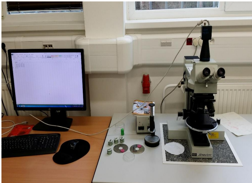
Figure 5.5 ARTCAM 300MI Microscope and Jenavert Microscope PA HD connected with a PC in Laboratory of CULS, Faculty of Engineering, Department of Material Science and Manufacturing Technology
