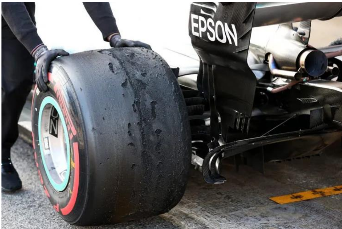
Obrázek 15: Blistering, zdroj: https://suspensionsecrets.co.uk/tyre-failure-graining-tearing-blistering-and-wearing/
