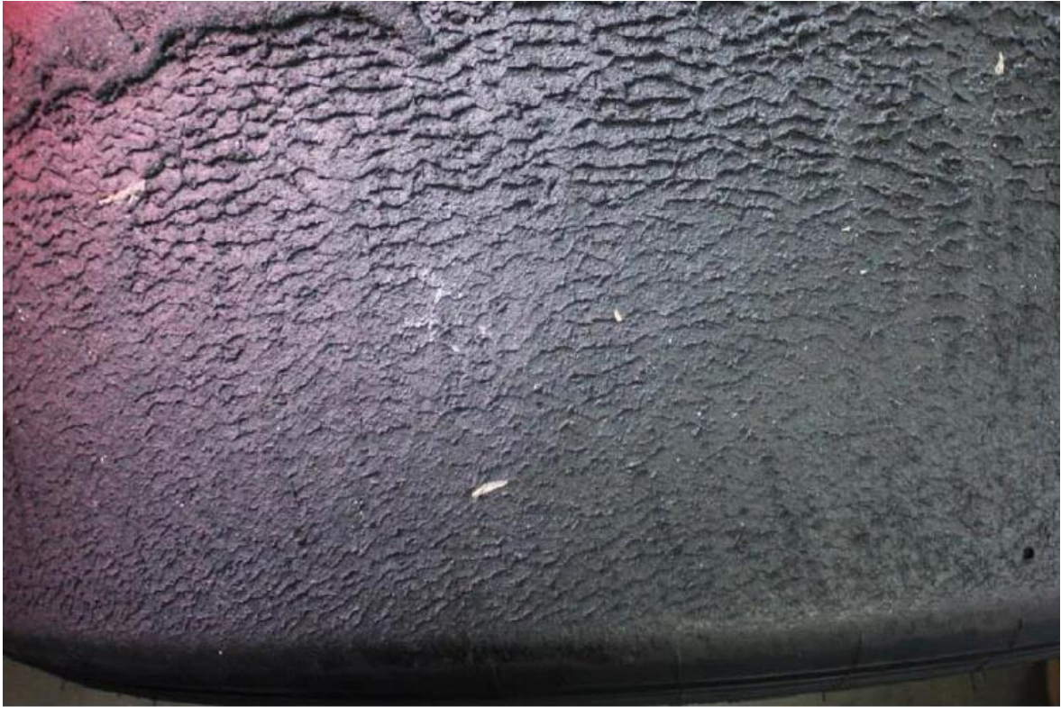
Obrázek 14: Graining, zdroj: https://suspensionsecrets.co.uk/tyre-failure-graining-tearing-blistering-and-wearing/
