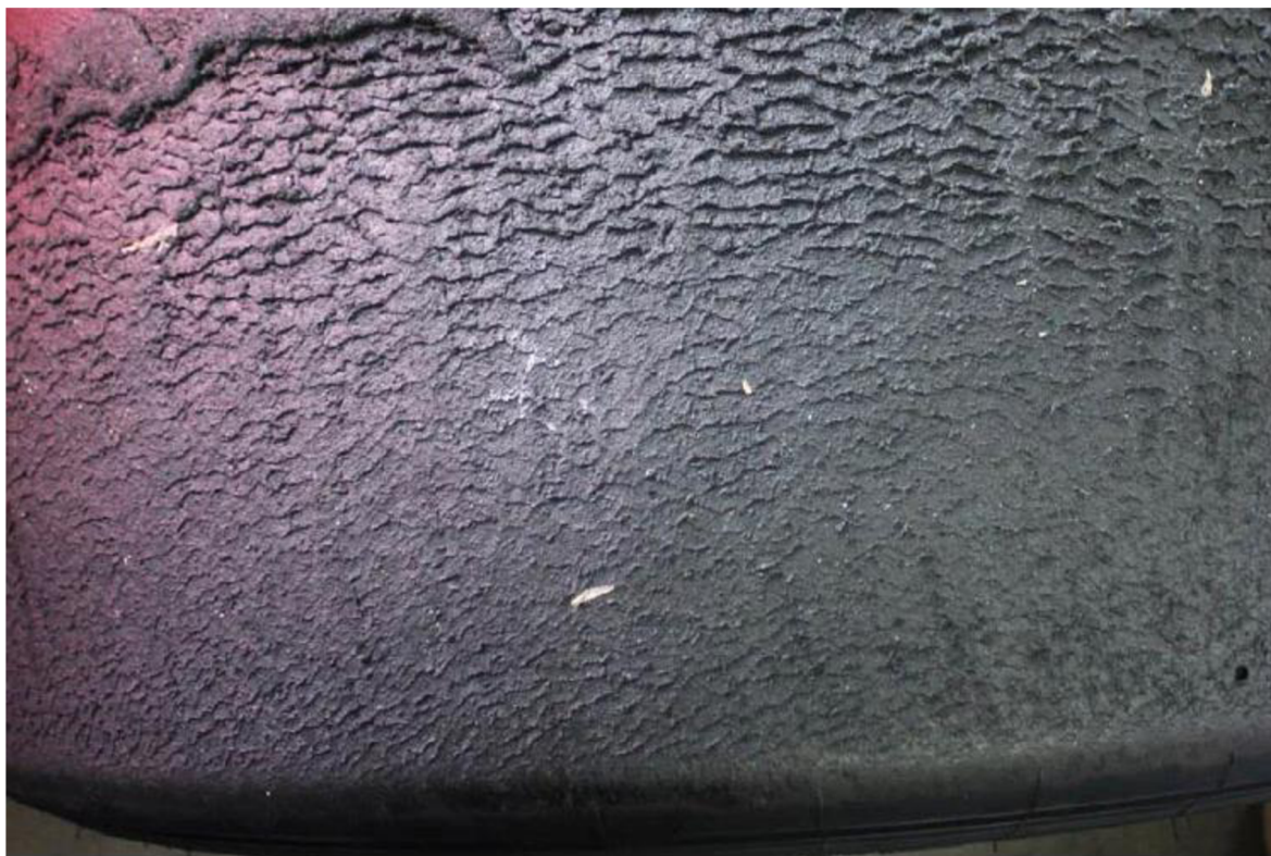
Obrázek 14: Graining, zdroj: https://suspensionsecrets.co.uk/tyre-failure-graining-tearing-blistering-and-wearing/
