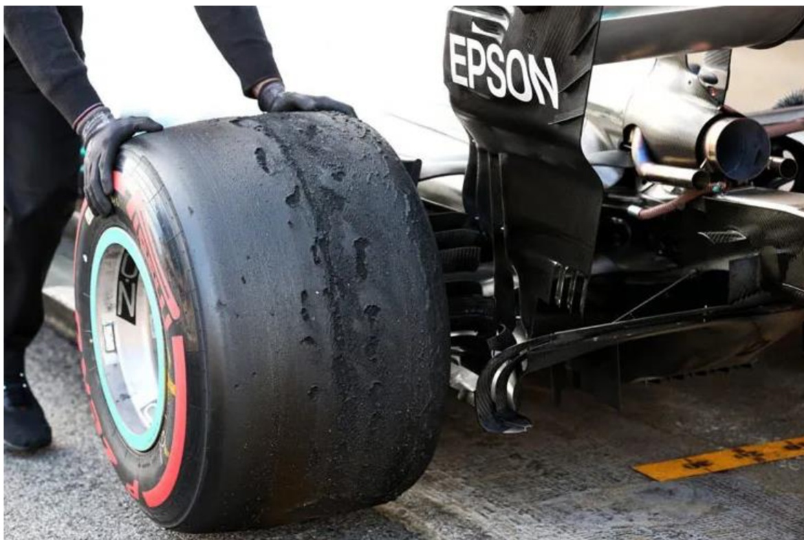
Obrázek 15: Blistering, zdroj: https://suspensionsecrets.co.uk/tyre-failure-graining-tearing-blistering-and-wearing/
