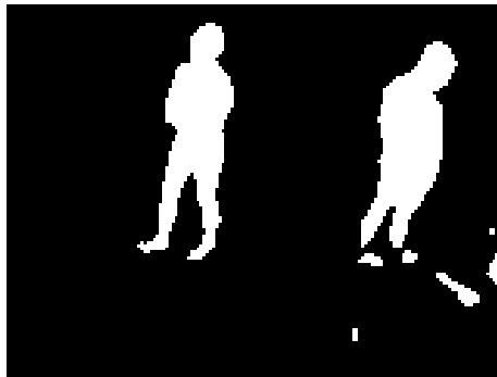
Figure 5.2: Example of thermal binary image after applying the adaptive mean thresholding.
