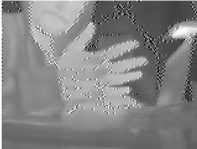
Figure 4.4: Illustration of artifacts after reconstruction back to Y16 format when using experimental method raw_over_rgb .
