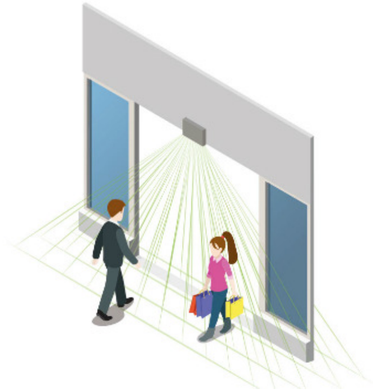
Figure 2.2: LIDAR based device for counting people entering and leaving through a doorway. (Source: [2].)
