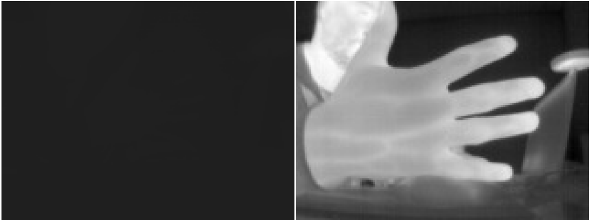
(a) Raw Y14 mode, no adjustments, pure data (b) Raw Y14 mode, linear AGC applied
