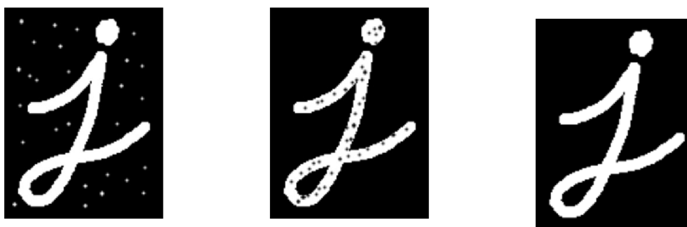
(a) Original noisy image suitable for opening. (b) Original noisy image suitable for closing. (c) Result image without noise.
