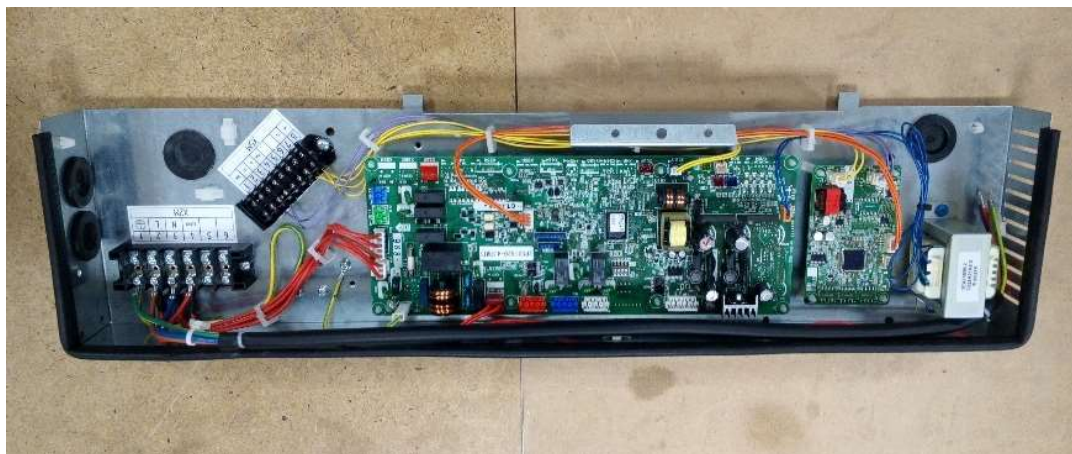
Obr. 2-6 Switchbox jednotky Alpha Hybrid [12]
