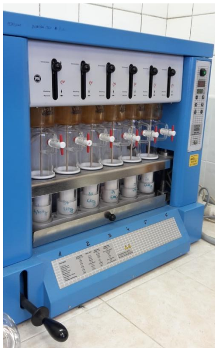
Figure 11 Soxtec apparatus used for fat extraction.
