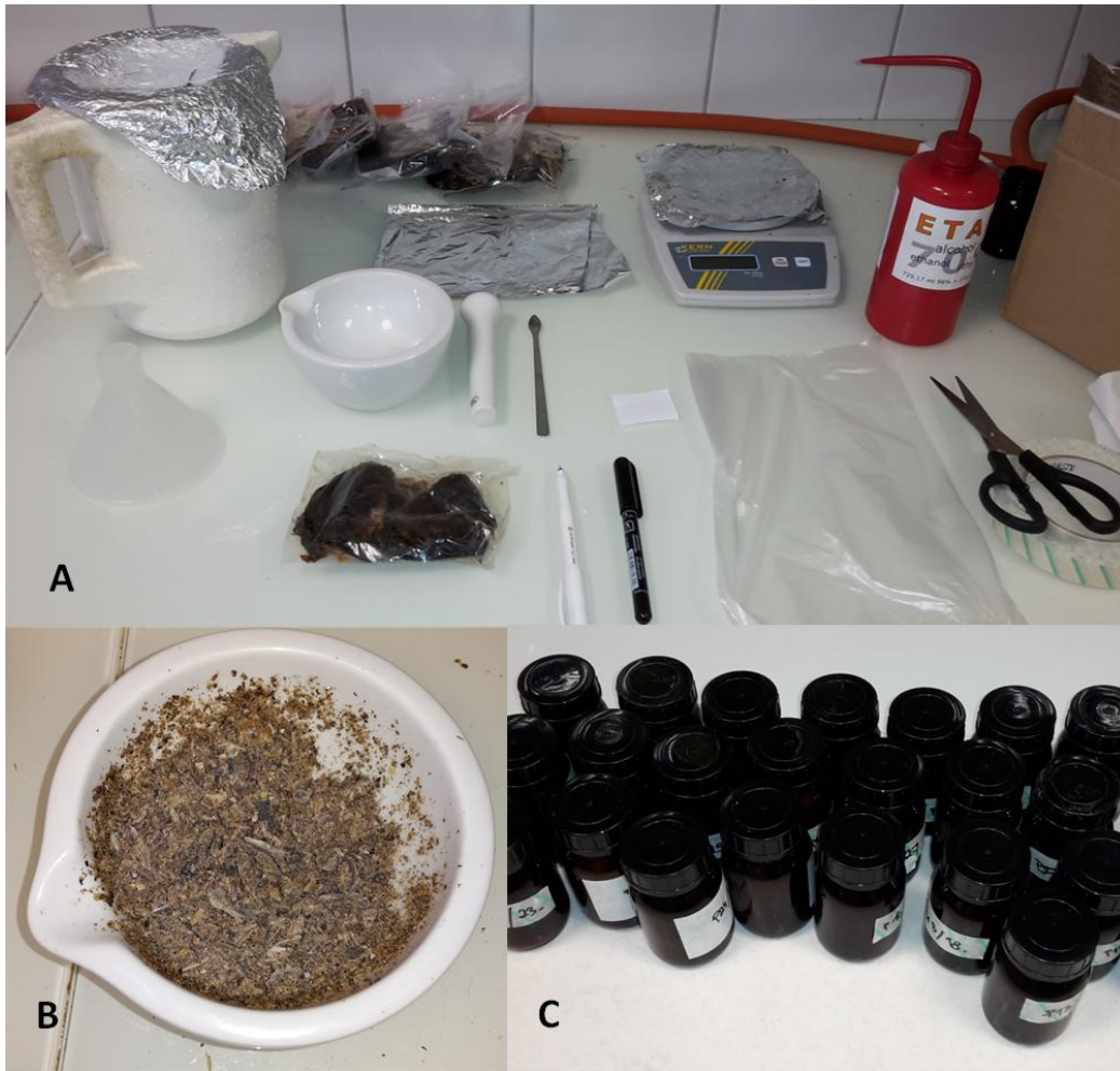
Figure 10 Sample preparation, prior to extraction. A – Laboratory equipment used, B – Homogenate obtained, C – Amber storage bottles.
