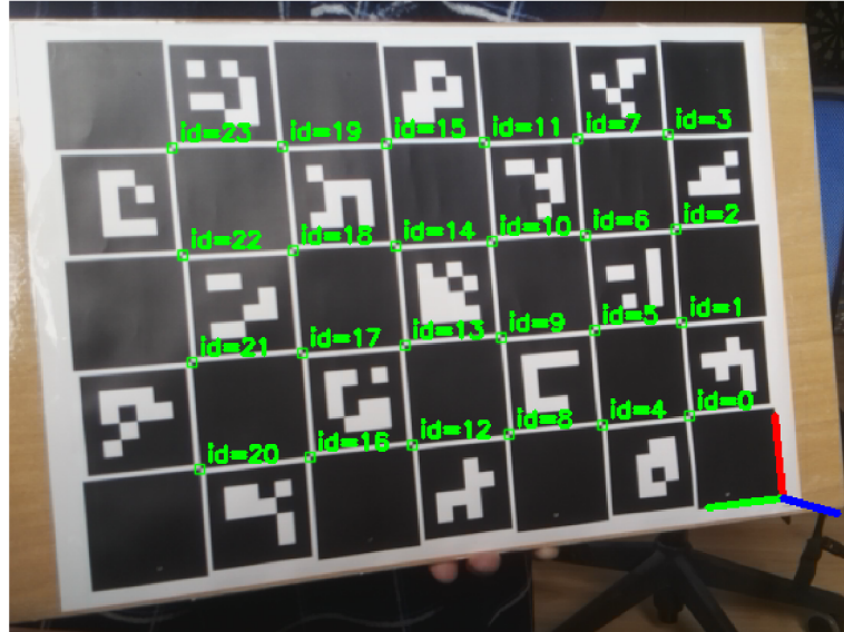
Figure 3.2: A projection of axes and corner IDs on the detected ChArUco board
