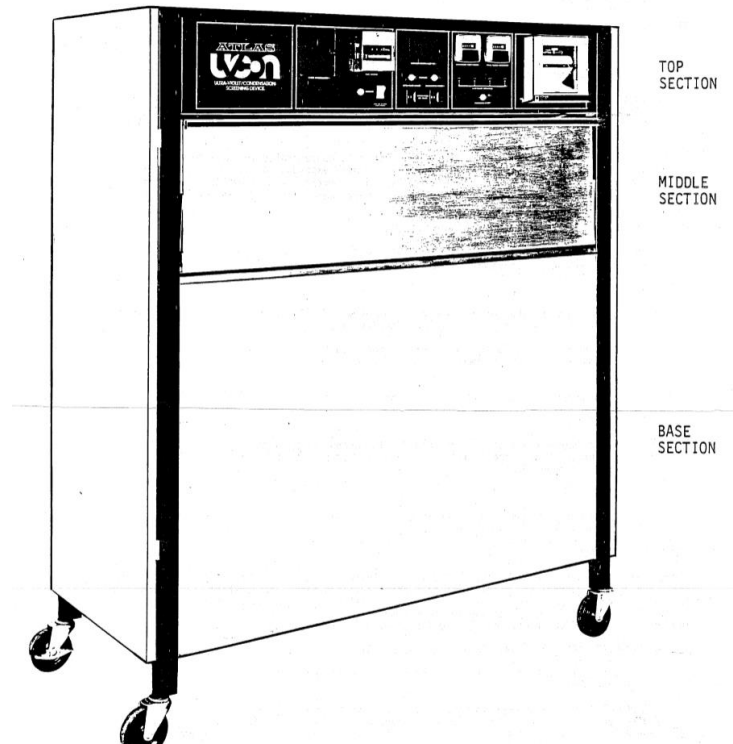
Figure 7: Atlas weathering machine [13]
