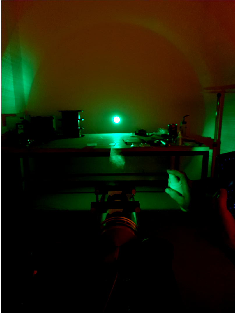
Fig. 8.7: Usage of spray to make propagation of beam visible.
