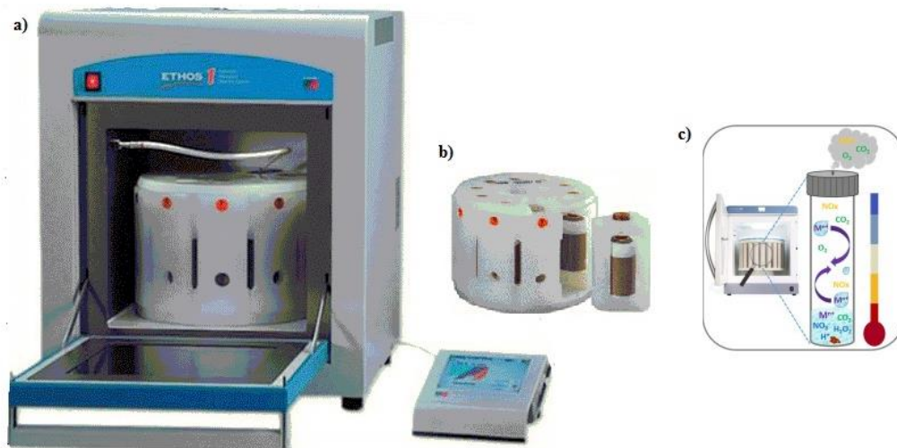
Figure 3 - Ethos 1 (MLS, Germany) - microwave-assisted wet digestion system: a) an appearance of apparatus, b) detail of inner rotor, c) detail of inner process inside of tube.
