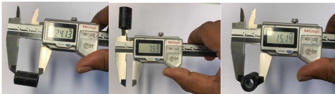
Figure 54: Measurement using vernier caliper
