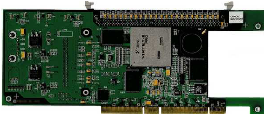
Figure 5.1: Front side of COMBO6X card
