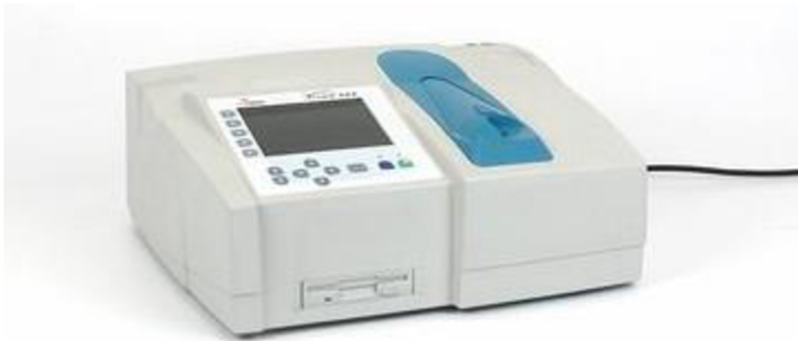
Figure 15 Spectrophotometer (Hach Lange Xion 500 LPG385) (Profcontrol GmbH 2022)
