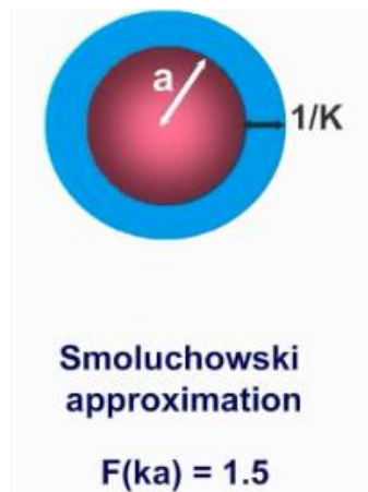
Fig. 17 – The scheme of Henry's function for aqueous media, where a represents the radius of the particle and \kappa^{-1} the layer of the electric bilayer [98].
