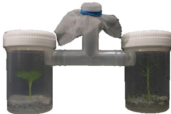
Figure 10. Vial system developed for performing larval feeding choice experiments.
