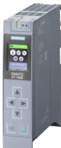
Obr. 23: PLC s CPU rady S7-1500 [10]
