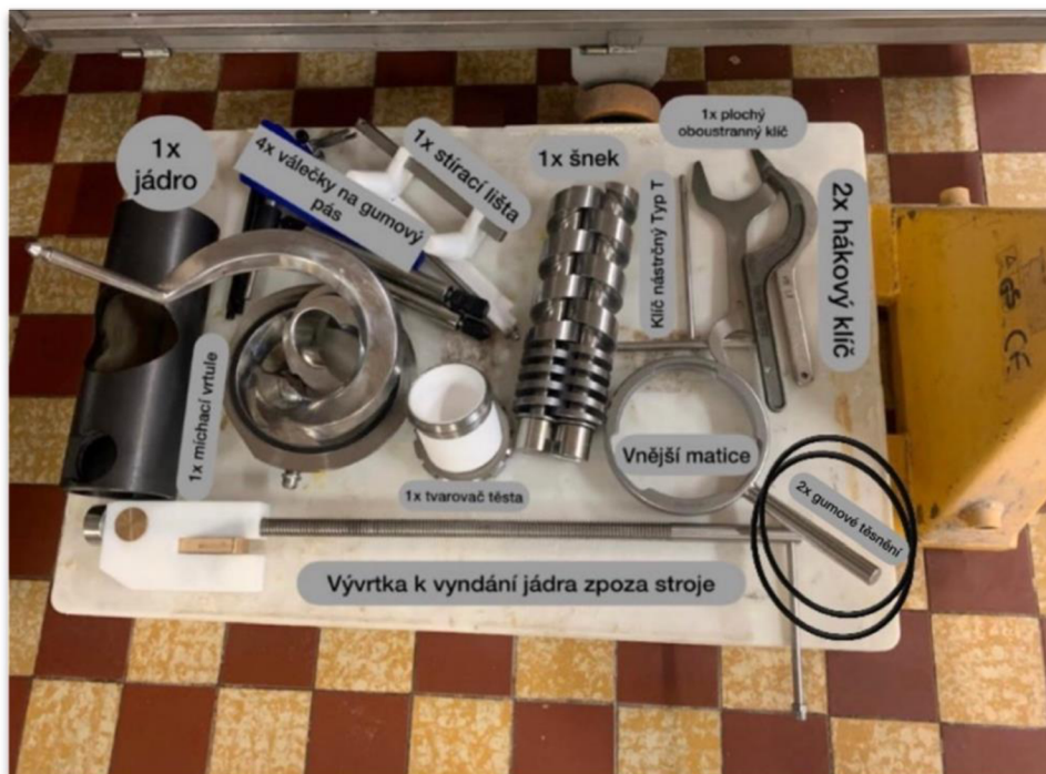
Figure 19: Placement of technical components on the pallet
