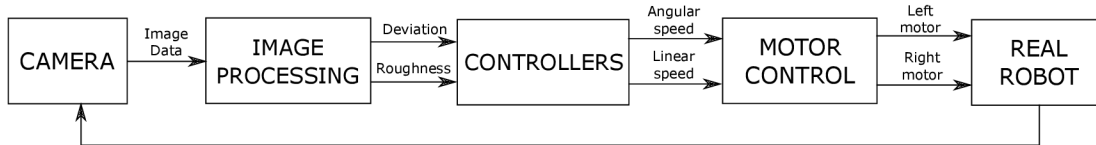
Fig. 8.1: Control diagram of modular code
