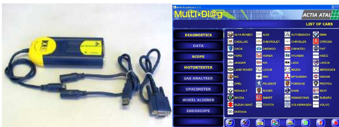
Obr. 3.11 – ATAL Multi-Di@g Access se software
