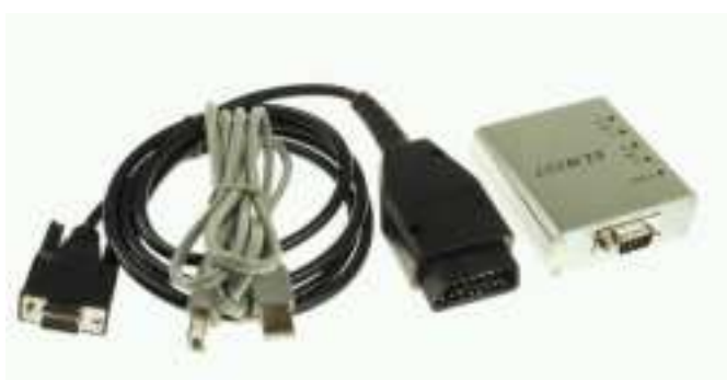
Obr. 3.5 – Interface CAN ELM 327 s USB
