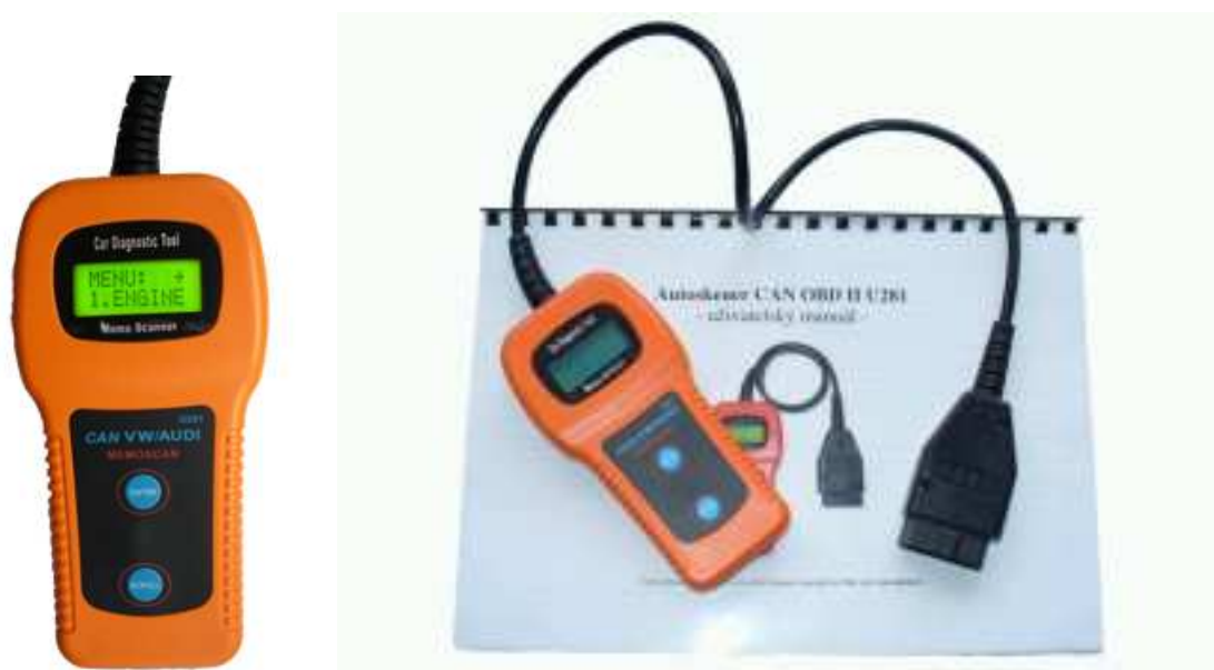
Obr. 3.7 – Autoscanner U281-CAN VAG
