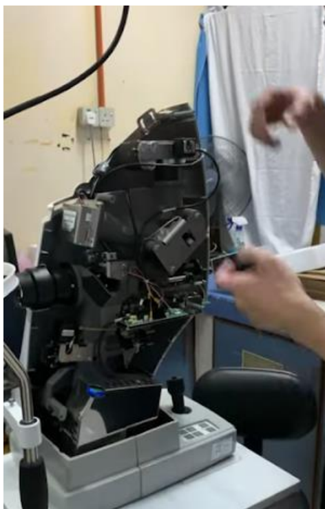
Obr. 2 - 17 servisovanie fundus kamery Zeiss [22]
