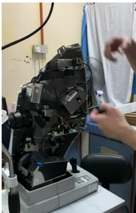
Obr. 2 - 17 servisovanie fundus kamery Zeiss [22]
