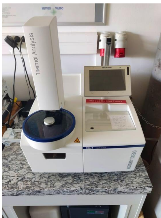
Obr. 3.8 Termogravimetr TGA2 Mettler Toledo
