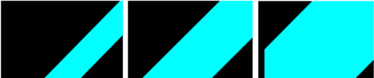
Figure 27: Illustration of moving bars stimuli. Left: 300 \mu\text{m}/\text{s} , 600 \mu\text{m} wide; Center: 562 \mu\text{m}/\text{s} , 1125 \mu\text{m} wide; Right: 990 \mu\text{m}/\text{s} , 1980 \mu\text{m} wide.
