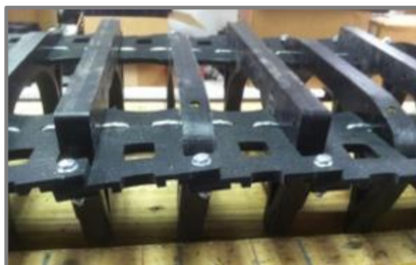
Obr. 29 Pás Adair Pro Series pro vozidla Argo [39]
