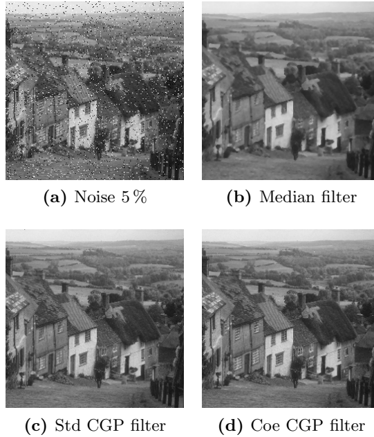
Fig. 5. Comparison of images filtered by median filter (b), the best filter evolved using the standard CGP (c), and CGP with coevolution (d)
