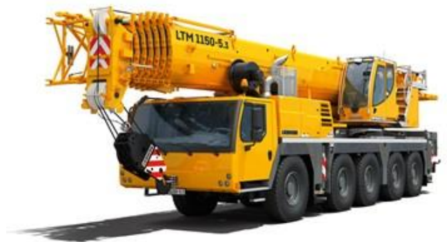
Obr. 47: Autojeřáb LIEBHERR LTM 1150-5.3 [33]
