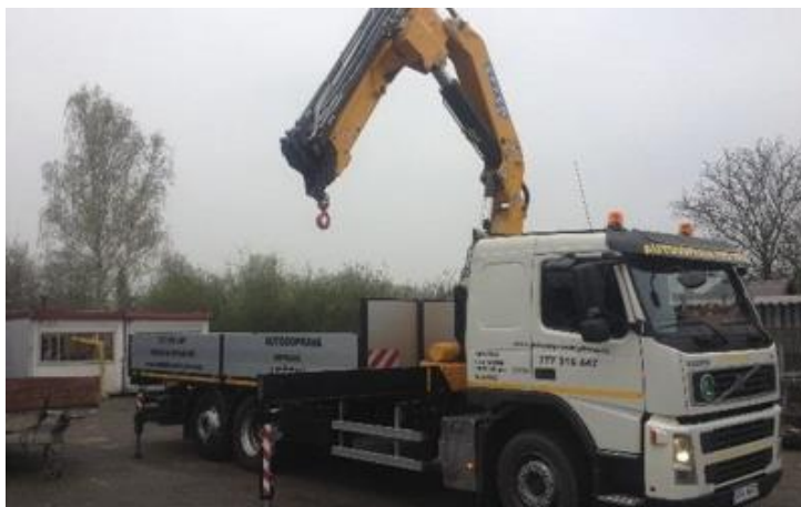
Obr. 68: Valník Volvo 370 s hydraulickou rukou Effer 325 4S [44]
