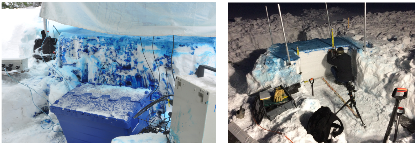
Figure 6.6: Left: Kubová Huť (Forest site) from outflow side with temperature sensors. The fiedler logger is located in the blue box. Photo credit: R. Juras. Right: Post experimental snow pit at the Luisino Údolí. Photo credit: J. Blöcher
