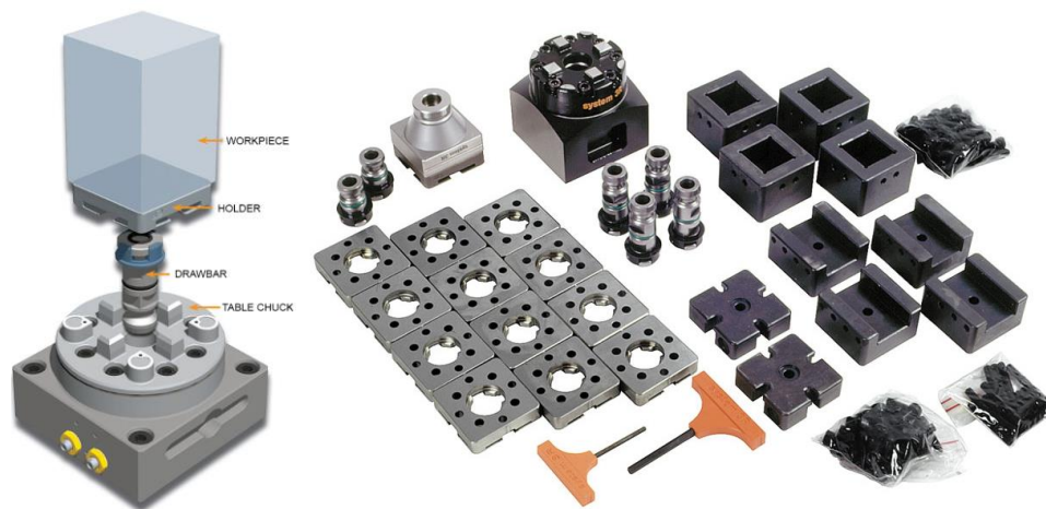
Fig. 4.4 3R Macro system (left), 3R Macro clamping kit from GF Machining solution (right) [24,26].
