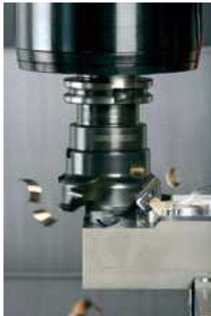
Obr. 4.2 High-speed spindle in a cutting process [8,10].
