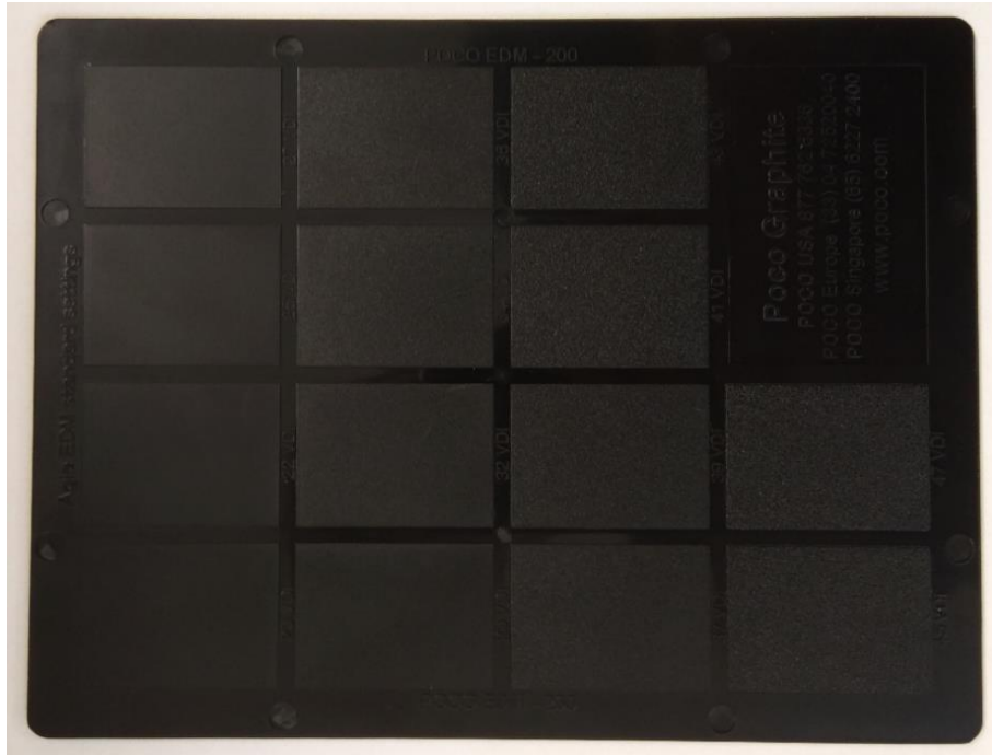
Fig. 1.23 VDI surface roughness plate from graphite supplier POCO graphite
