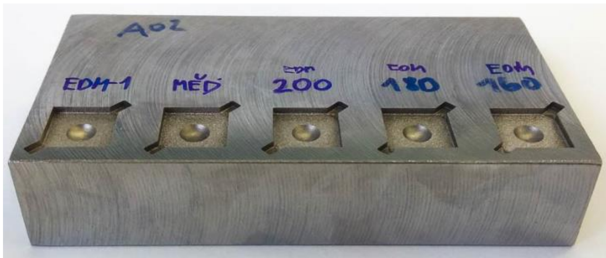
Fig. 7.13 EDMed cavities ready for another measuring process.
