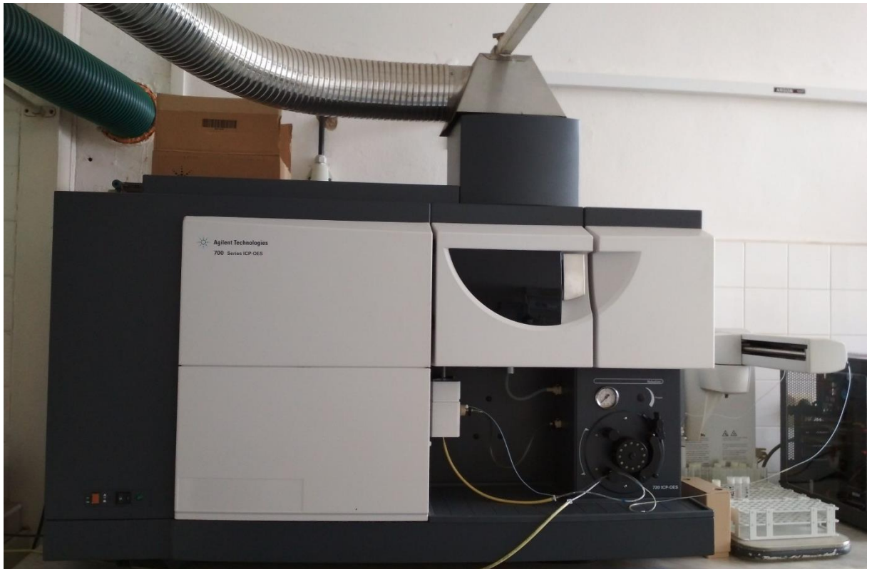
Figure 12: Inductively coupled plasma-atomic emission spectrometry (ICP-OES Agilent 720, Agilent Technologies Inc., USA). Source Kateřina Vejvodová
