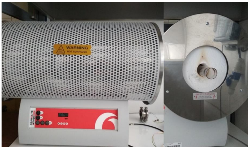
Figure 9: Pyrolytic furnace Carbolite 301 (Carbolite Gero, Great Britain). Source: Kateřina Vejvodová
