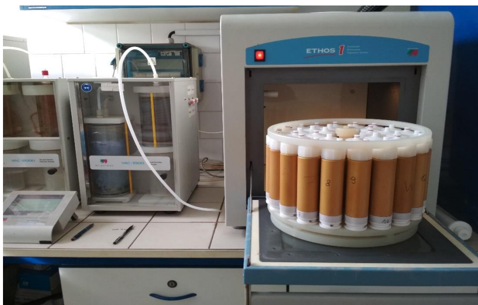
Figure 10: Ethos 1 (MLS GmbH, Germany) microwave-assisted wet digestion system. Source: Kateřina Vejvodová
