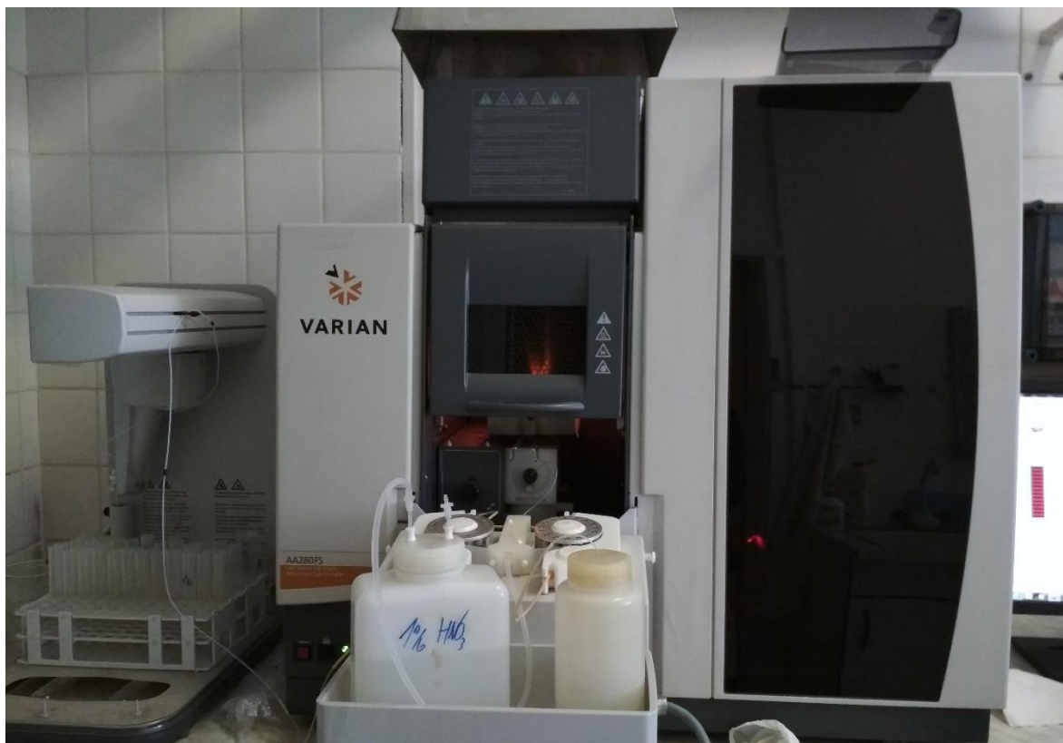
Figure 11: Flame atomic absorption spectrometry Varian 280 FS (F-AAS, Varian, Australia). Source Kateřina Vejvodová
