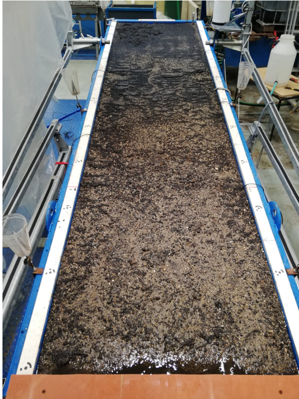
Fig. 3.2: Rainfall Simulator (RS) in the laboratory of the Faculty of Civil Engineering of the Czech Technical University in Prague (CTU)
