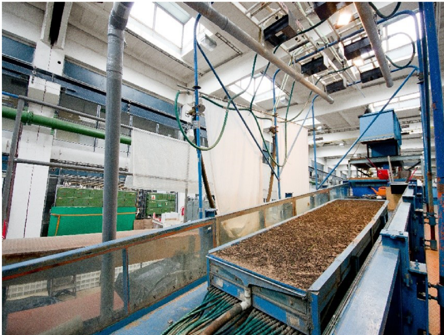
Fig. 3.1: Rainfall Simulator (RS) in the laboratory of the Faculty of Civil Engineering of the Czech Technical University in Prague (CTU)
