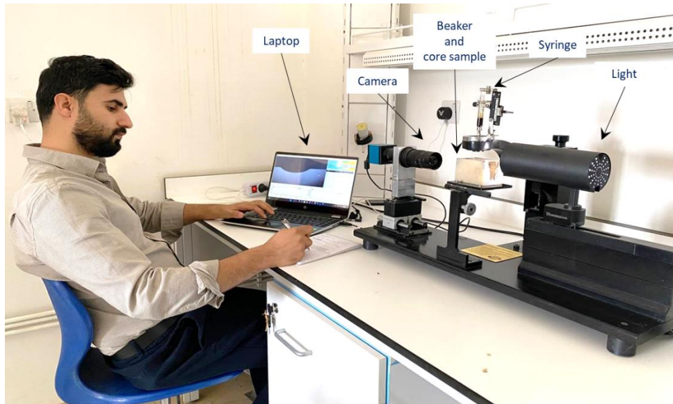
Figure 23 Contact angle measurement setup.
