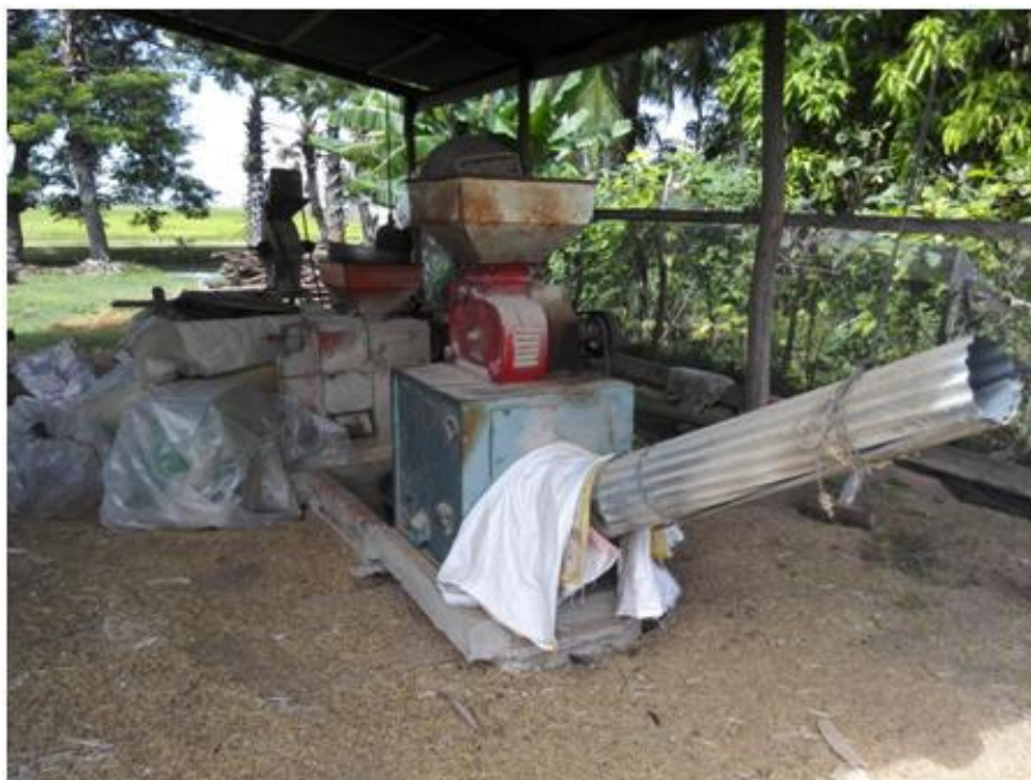
Figure 18: Village miller's rice milling machine
