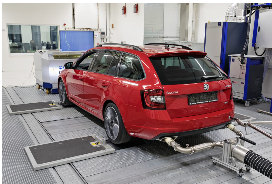
Fig. 3.20. WLPT Vehicle Test Procedure [Skoda Auto Employee Portal]
