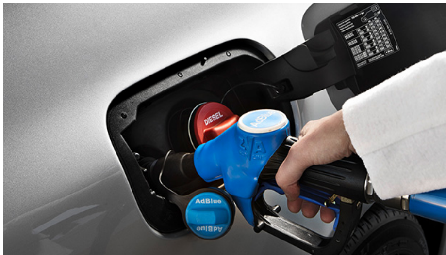
Figure 3.33: The fluid cleans diesel exhaust fuels and effectively converts it into harmless water and nitrogen that is exhausted. [40]
