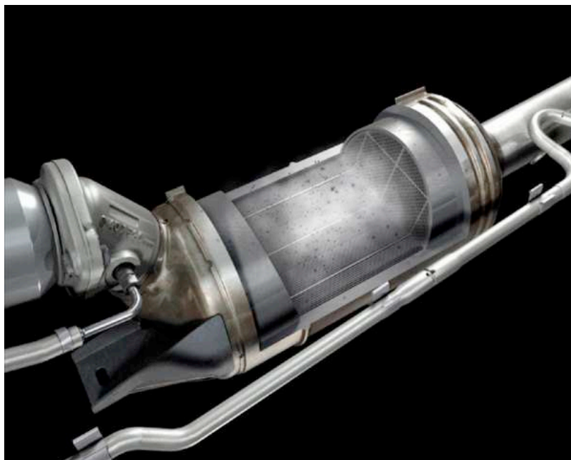
Figure 3.37: An opened DPF from a light commercial vehicle. [9]
