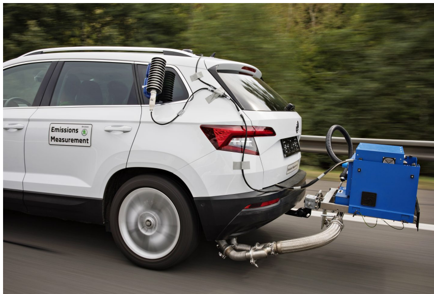
Figure 3.25. Emission are being measured with emission portable measurement system [Skoda Auto Employee Portal]
