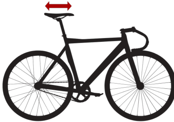
Figure 2.4: Saddle setback is the horizontal position of the saddle with respect to the bottom bracket.
