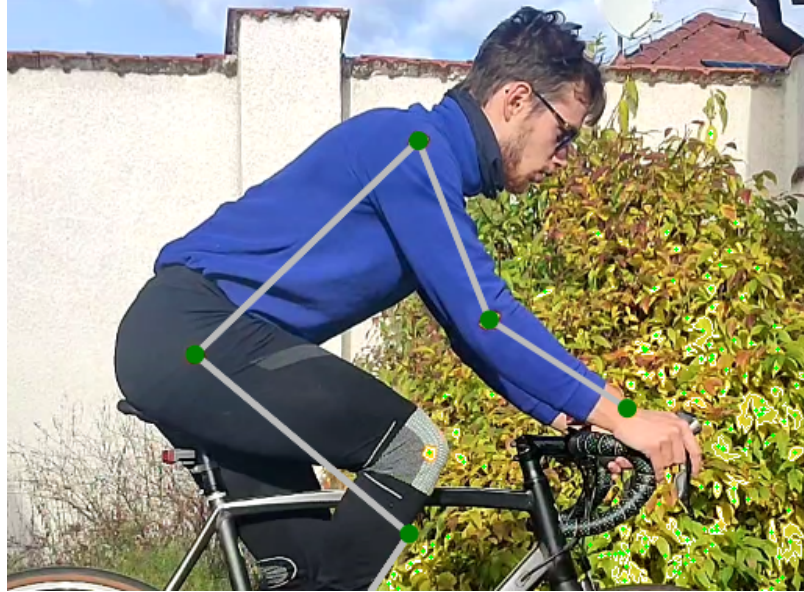
Figure 3.4: Example of a failed localization of the markers. The leaves in the background have similar color to the markers and the knee marker is therefore not localized correctly. The location of the markers is show as the green dots.
