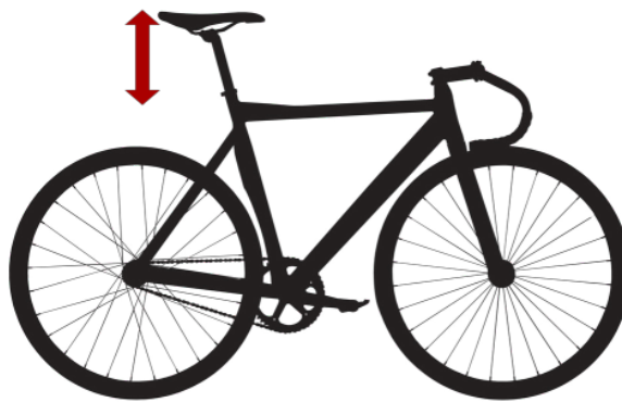
Figure 2.1: Saddle height measures how high is the saddle compared to the bottom bracket.
