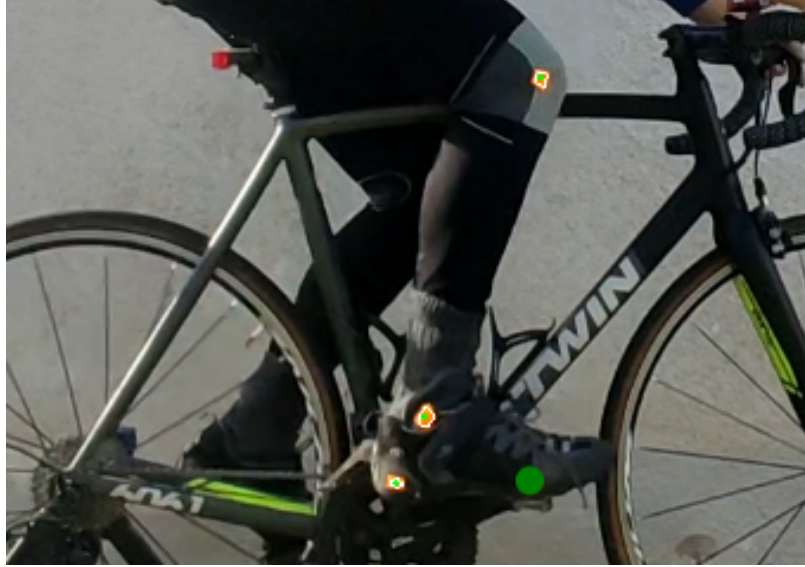
Figure 3.2: Closeup of the localization of the markers. The single localized foot marker is highlighted in green. The contours of the thresholded regions are highlighted in white. The centroids of the contours are highlighted by small green cross.
