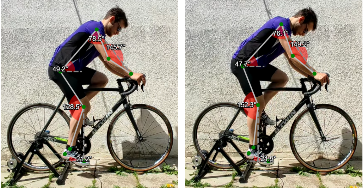
Figure 8.1: Screenshots of the videos with saddle heights of -3.5 cm (left) and +2.5 cm (right) with the keypoint predictions and angles overlaid on the video. Both screenshots show the knee angle at the bottom of the pedal stroke.
