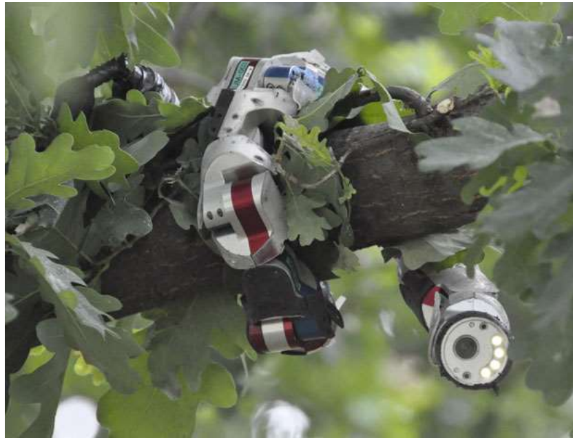
Figure 4 An example of 16-joint modular snake robot [01]
