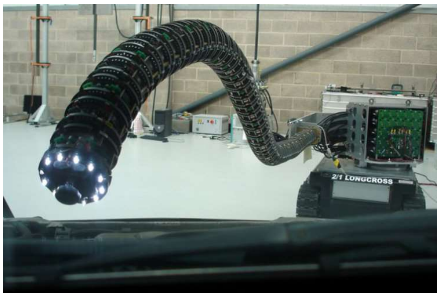
Figure 7 The snake arm by OC Robotics is being used to explore a vehicle
