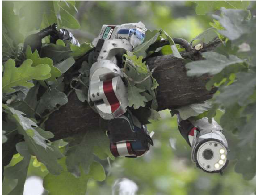
Figure 4 An example of 16-joint modular snake robot [01]
